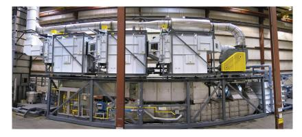
Munters was asked to design a compact, highly efficient heat exchanger and burner package that would work with a Selective Catalytic Reduction (SCR) system for the reduction of nitrogen oxides (NOx). The heat exchanger was required to be capable of handling widely varying system air flow rates and needed to operate using either natural gas or propane.
